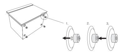
■ Carefully place the appliance on its back and screw the four feet into the holes provided (see illustration).
